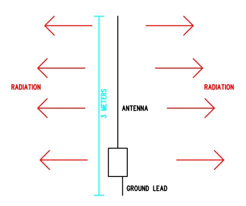
Explanation of Part 15.219 , only the allowed 3 meter area is supposed to radiate.
