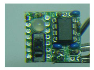
To install the AM1000T yourself you may need to solder connectors and wires, do not do this if you don't feel competent. Place the AM1000T as shown into the 14 pin pattern on the main AM1000 printed circuit board. Solder the 14 pins on the bottom of the AM1000 board. The Solder the 2 sense wires as shown. The left wire goes to the bottom pad of C18 and the right wire goes to the top pad of C35. The AM1000T should then function as above. If it doesn't check the sense wire connections.
