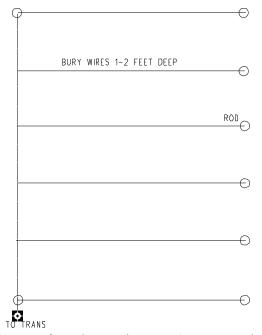
The type of trench ground system above can work well with sandy/dry soil.
