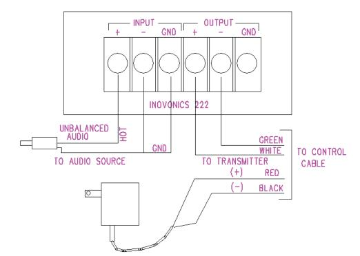
Here is the 222 wire diagram showing the input in the unbalanced method.
