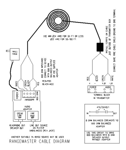
Wire diagram for the transmitter system. There are two terminal blocks, either can be used. Not shown is the cable shield drain connection, connect it to the GND terminal on the terminal block in the transmitter.
