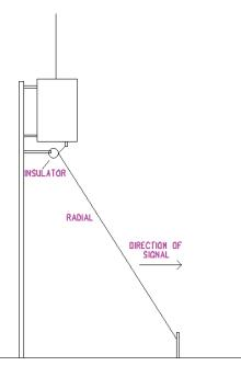
We have referred to buried radials earlier. In general for a radial to be effective the length should be more then the height of the antenna tip is from the ground. A radial is just a wire going from a center ground rod outward.
