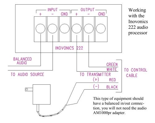
Connections for balanced audio in. These connections should be the same for other audio processors.
