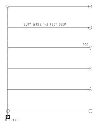
The type of trench ground system above can work well with sandy soil.
